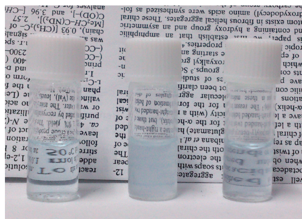
Figure 4. Photograph of [Cu(L-AlaC 12 OH) 2 ] (left), [Cu(D-AlaC 12 OH) 2 ] (right), and [Cu(D,L-AlaC 12 OH) 2 ] (center).
